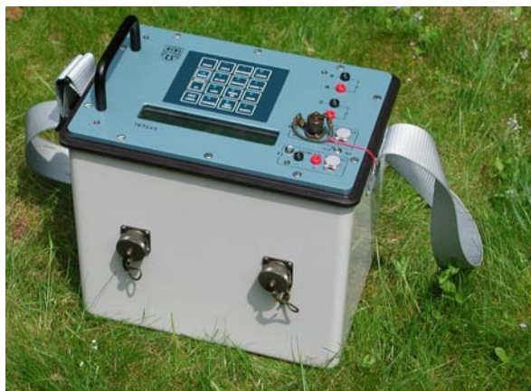
SYSCAL R1 Plus Switch, 24, 48, 72 600V, 200W, 2.5A
