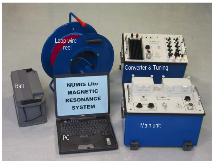
Fig 1: The NUMIS Lite Magnetic Resonance Sounding system for water investigations down to approximately 50m depth.
