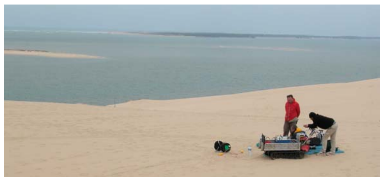
Fig 2 : Sketch (on top) showing the locations of the MRS soundings (stations A, B, C), and two pictures of the Pyla dune (top right) and of the location of station B with NUMIS Lite equipment placed on a caterpillar wheel trolley for an easier transportation on the sand (right).
